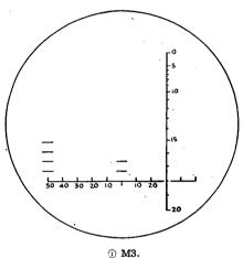
FIGURE 11.—Reticles, binocular.
